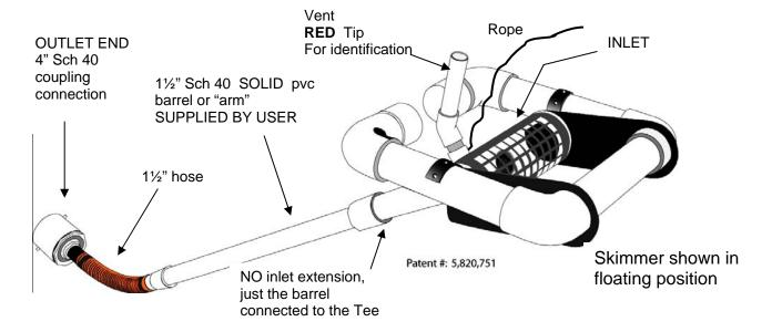
2. Glue the 1½" Sch 40 barrel pipe to the 1½" white coupling on the hose.
