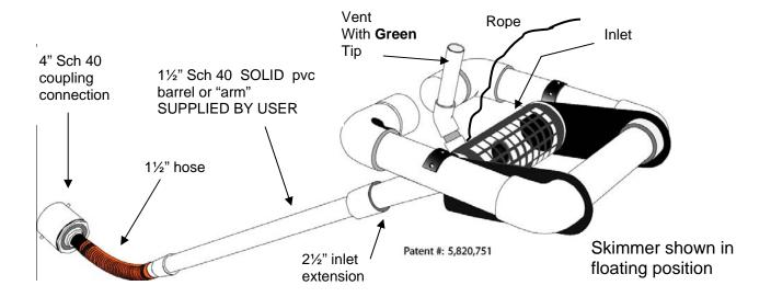
2. Glue the 6' long 11/2" sch 40 barrel to the 11/2" grey coupling on the hose.
