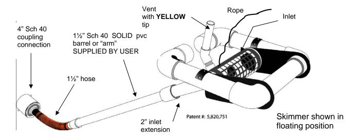
2. Glue the 6' long 1½" sch 40 **barrel** to the 1½" grey coupling on the **hose**.
