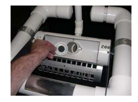
If a pool of water is to be provided, install the support under the skimmer inlet as shown on the erosion control plans. It is recommended that the hose connection to the pipe through the dam be <u>low enough that the whole pond can be drained using the skimmer</u> even if a pool of water is to be provided. Doing this will avoid using a pump to drain the very bottom of the pond.
