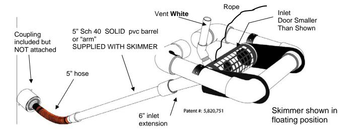
2. Glue the 10' long 5" sch 40 barrel to the 5" white coupling on the hose.
