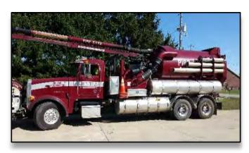
Combination Sewer Truck with 1,500 gallon water tank
