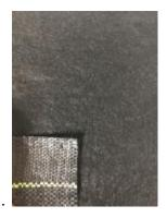
DeWitt Pro 5 Weed Barrier is a woven, needle-punched polypropylene fabric for commercial grade weed control. Specified by leading architects, the fabric is designed to allow air, water, and nutrients through. The fabric will not rot or mildew, and is formulated to resist uv degradation.
