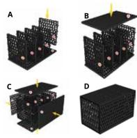
Figure 2 Follow these steps to assemble a 5-plate R-Tank<sup>HD</sup>®
