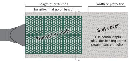
Culvert outlet protection – plan view
