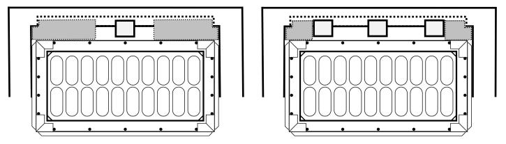
The SplashGuards are cut down to fit the curb throat opening as shown above. Please note that the intent of the SplashGuard is to divert the flow down the curbline into the StormSack BMP unit.
