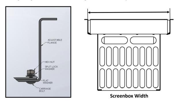
**4.** Loosen bolts as necessary and adjust sliding drop flanges to the required position and secure in place using a standard 7/16" socket wrench. Do not overtighten bolts.
