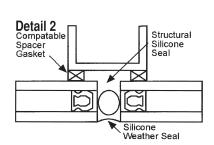
For insulating glass, the design must be changed to accommodate Figure 1 and Detail 2, unless a one component silicone secondary seal is used.
