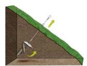
The first stage is where a load is applied to rotate the anchor into its loadlocked position. Elements of both load and extension are present.
