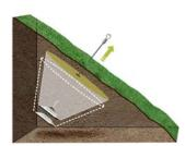
The second stage is where the anchor system is generating a frustum of soil immediately in front of the anchor. At this point load normally increases with minimum extension. The soil type will affect the overall extension.
