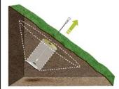
Caution: If the mechanical shear strength of the soil is exceeded, the residual load will decrease with continued extension as the anchor shears through the soil.
