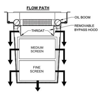
When stormwater enters the Fabco Screen Box, it passes through and over an optional oil boom that is placed around the top perimeter of the box. After this initial pretreatment, the water flows down through the protected bypass hood into the lower filtration chamber.
