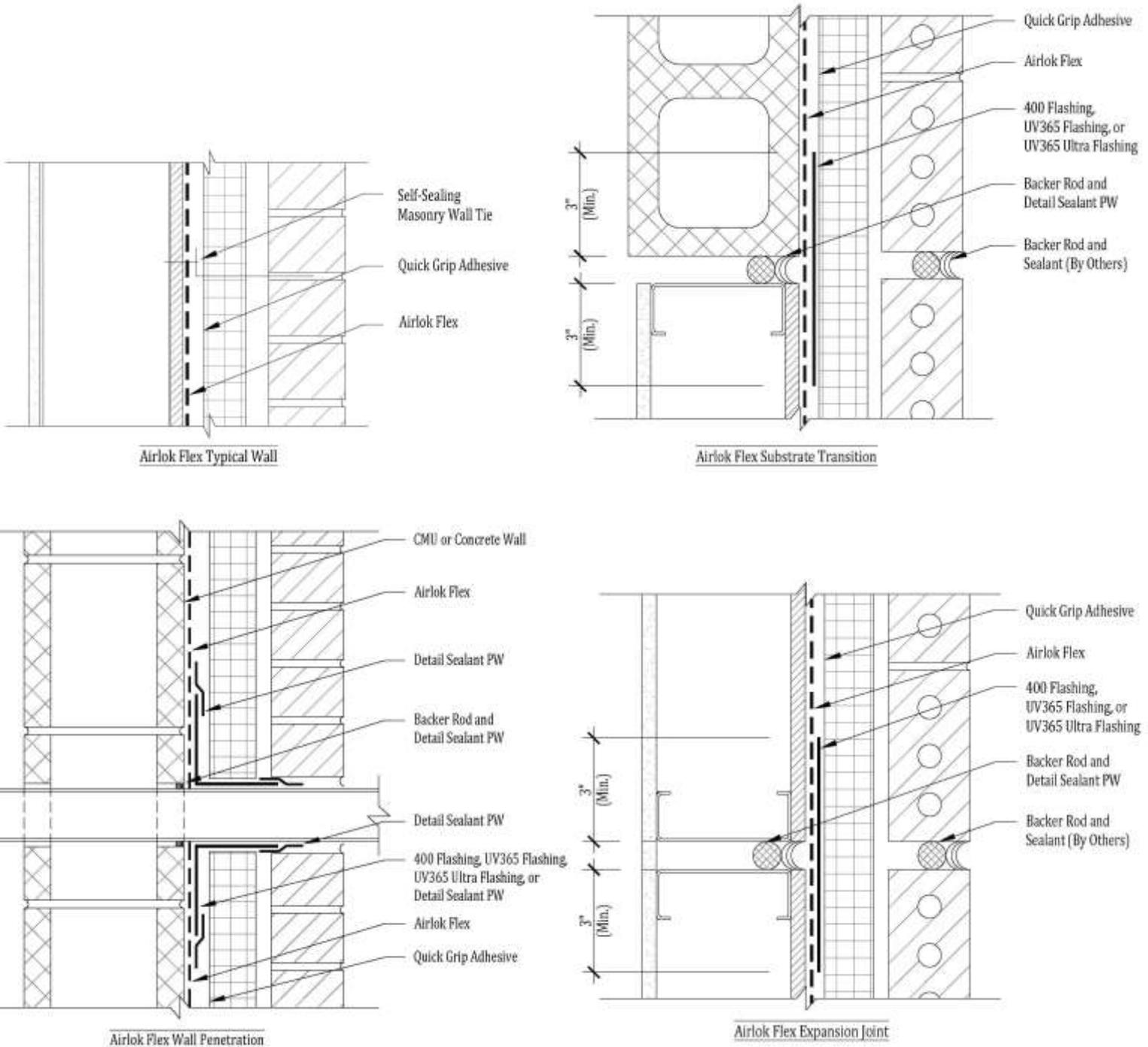
**Please Note:** Not intended to be full details. For full application detail on these configurations, see Polyguard Airlok Flex details or contact Polyguard Products.
