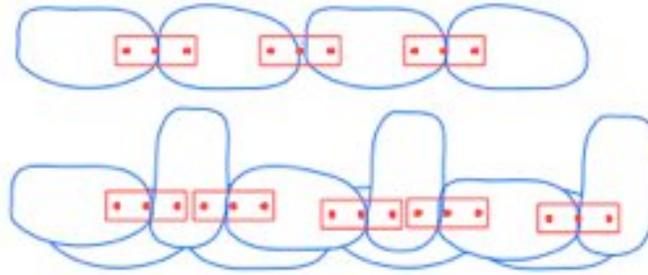
Fig. 3 Flex MSE Cross Section with Reinforcement
