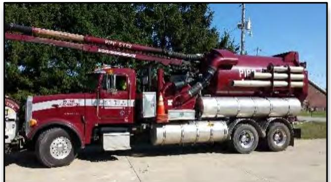
Combination Sewer Truck with 1,500 gallon water tank
