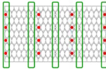
Fig. 1 For standard R-Tank<sup>LD</sup>® (4-plate) projects, attach small plates at locations with red dots. For R-Tank<sup>HD</sup>® and R-Tank<sup>SD</sup>® (5-plate) projects, attach small plates at locations circled in green.
