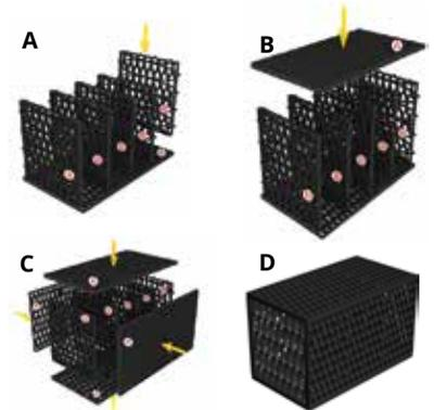
Figure 2 Follow these steps to assemble a 5-plate R-Tank<sup>HD</sup>®.
