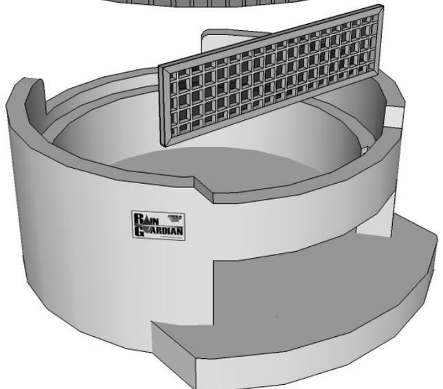
Steel reinforced monolithic concrete riser and base (1,030 lbs.)
