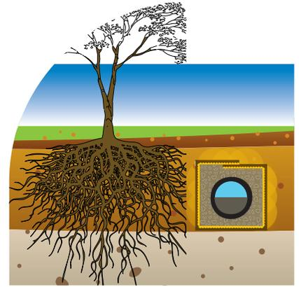
**Tree roots seek out air and moisture in the soil, causing expensive damage to underground infrastructure. BIOBARRIER'S unique geotextile design lends flexibility to surround infrastructure, extending the life of your investment**
