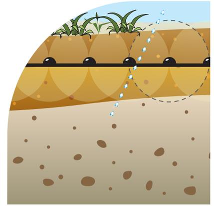
**Installed horizontally below three inches of stone/wood mulch, the BIOBARRIER weed control system blocks weeds using two layers of defense: chemical and physical.**
