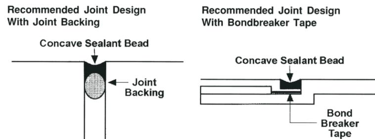
**Lap-Shear Joints should have a bead which is equal to, or greater than, the total anticipated movement.**
