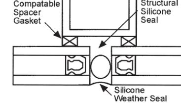
For insulating glass, the design must be changed to accommodate Figure 1 and Detail 2, unless a one component silicone secondary seal is used.
