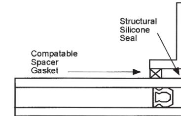
DETAIL #1 is commonly used in shop glazed applications where a glazing insert or split mullion is used. Care should be taken in applying the structural sealant to avoid direct contact with the insulating glass edge seal. The cure by-products are free to dissipate into the surrounding atmosphere and would not be entrapped in direct contact with the silicone I/G seal.
