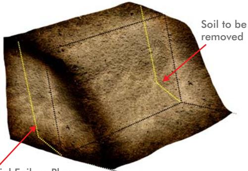
Potential Failure Plane
