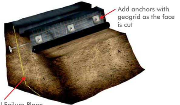
Potential Failure Plane
