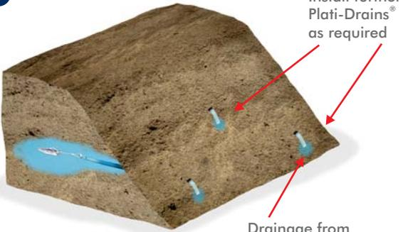
Install further Plati-Drains® as required
