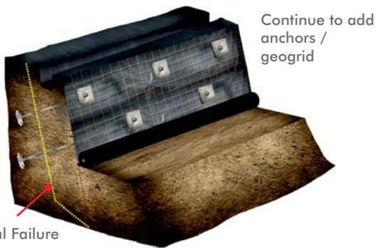
Potential Failure Plane
