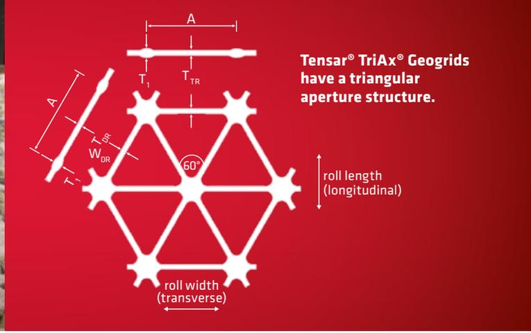
a geogrid with a very high junction efficiency (ratio of junction strength to ultimate tensile strength) to offer optimal rib-to-rib stress transfer. This meets the need to effectively and uniformly distribute loads for both paved and unpaved applications.
