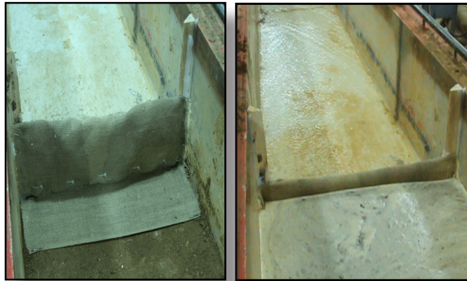
Shown Left to Right: WattleFence Before Testing, WattleFence During Testing.
